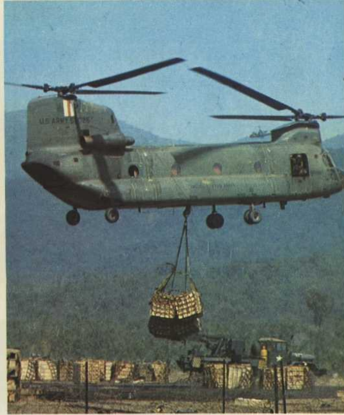
Aerial resupply is one of the jobs performed by the Chinook helicopter, carrying goods either inside or by sling load.
